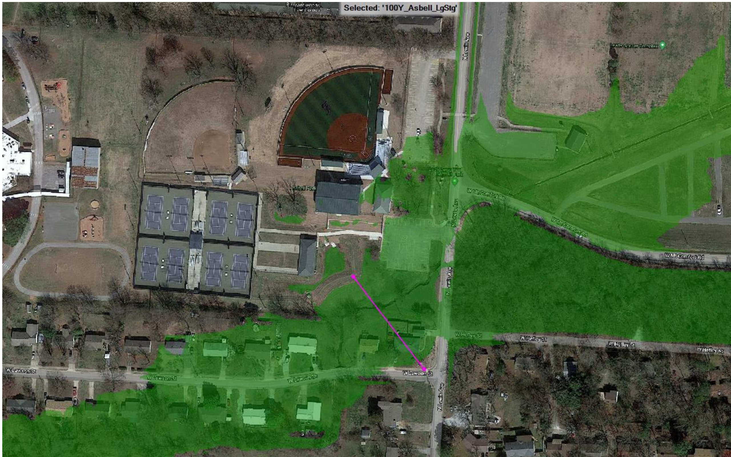
Figure 18. Large Storage Pond – 100-Year Lewis Storage.
