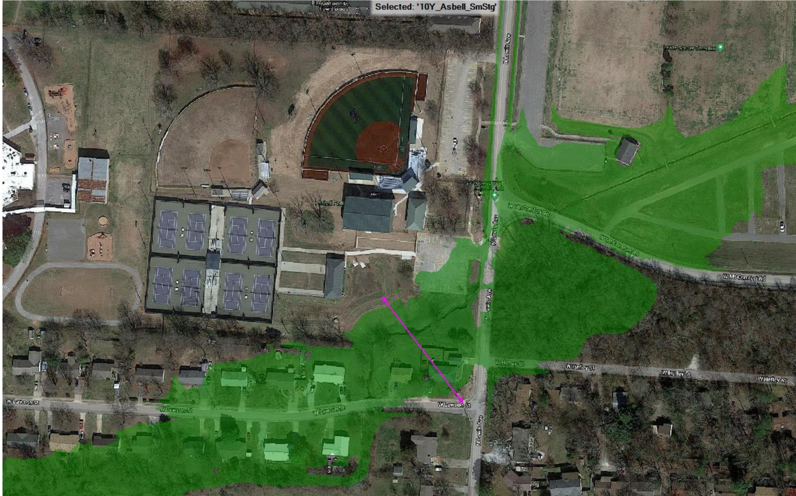
Figure 14. Small Storage Pond – 10-Year Lewis Storage.
